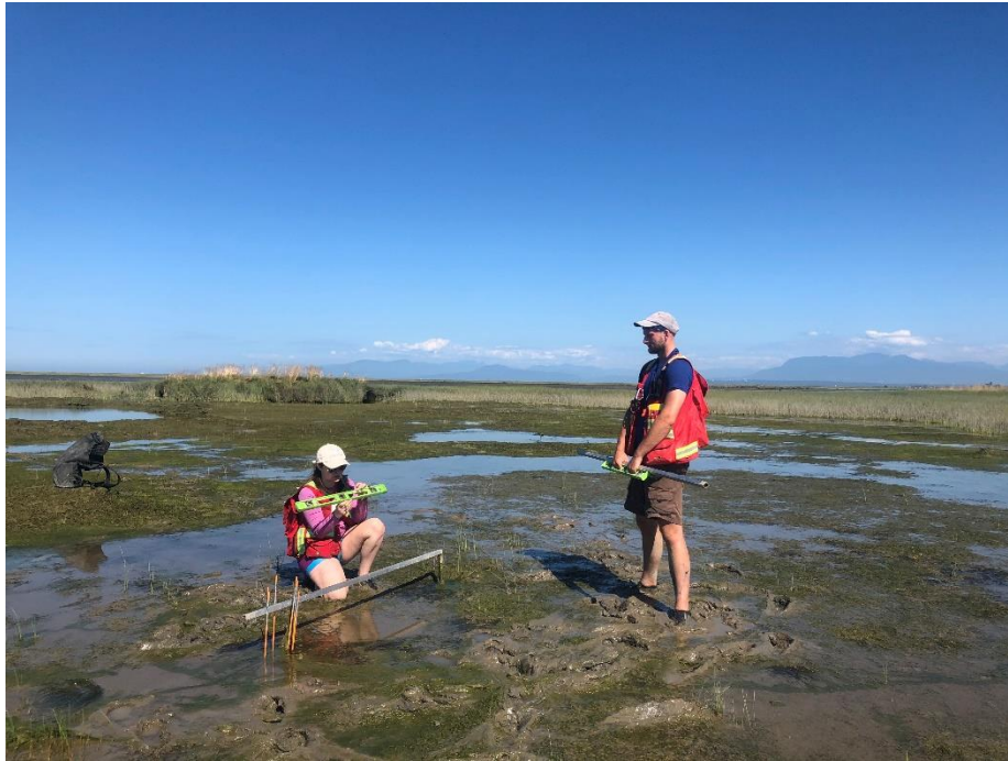
Roberts Bank WMA – Measuring sediment elevation at long-term monitoring station for marsh recession research.
